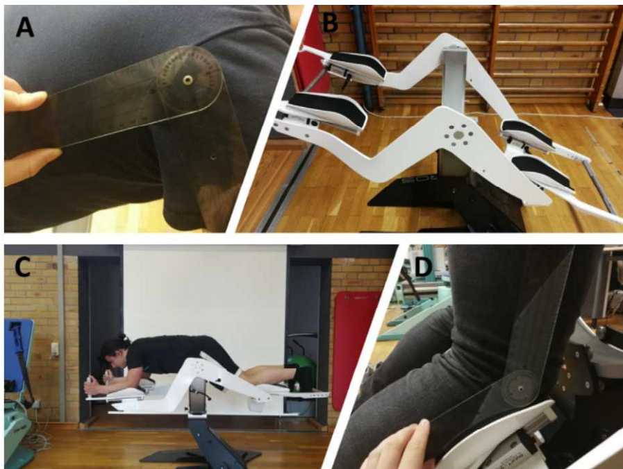
Fig. 2. (A) Torso–arm angle measurement using protractor, (B) Icaros device, (C) participant being familiarized with the device, (D) upper-to-lower limb angle measurement using protractor. [30].
