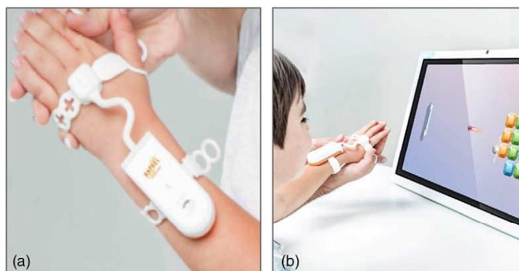
Fig. 11. Component of the virtual reality device developed for upper-limb rehabilitation in children with disabilities. [17].
